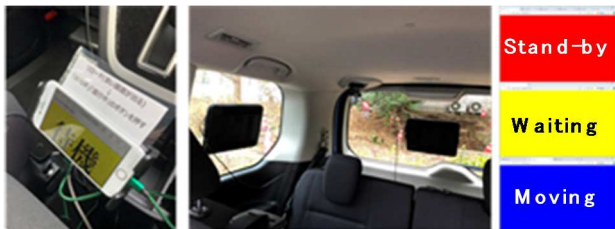
Figure 9 Operation status display system
